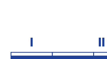
Lay the cut carpet tile "II" in the space in between.
